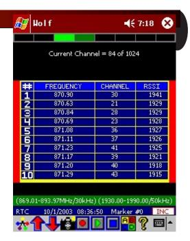
The data is stored in a compact proprietary binary format. The Wolf will store data as it received from the hardware, depending on the currently active screen. If the spectrum screen is currently active, spectrum data will be stored. If the access point screen is currently active, access point information will be stored.
